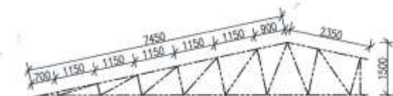
TRUSS 01c (5 No.) SCALE 1:50
